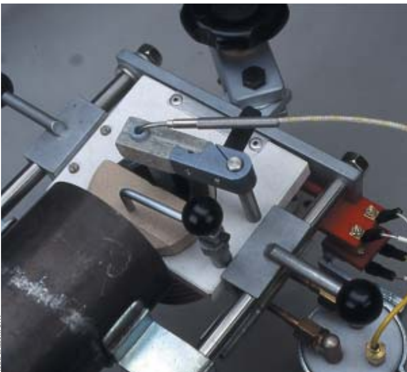
Close-up of crucible and flask on Galloni broken arm centrifugal casting machine
